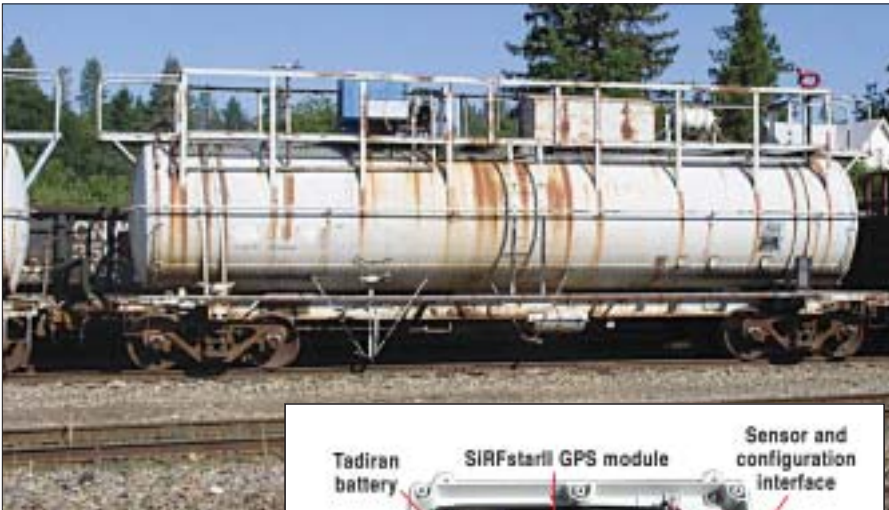
Figure 5. AXTracker mobile asset trackers are self-contained, battery-powered telemetry devices that can be attached to the outside of railcars, cargo containers, or trailers. The units send multiple daily transmissions of GPS location as well as other data via the Globalstar Satellite Network.
