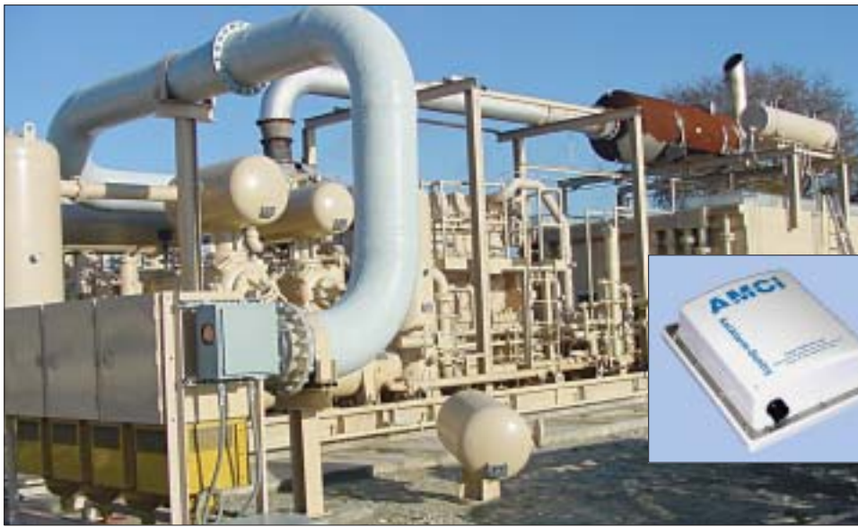
Figure 2. The SatAlarm-Sentry, shown here monitoring a gas pipeline compressor unit, provides early warnings of out-of-bounds conditions in remote installations. Powered by a hybrid lithium battery pack, SatAlarm devices offer up to 20 years of service between battery replacements.
