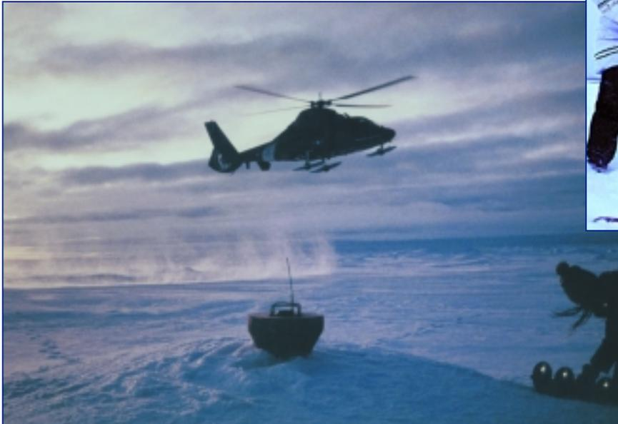
*Oceantronic's GPS/ice buoy being retrieved by helicopter to the Arctic for use in experiments measuring wind, temperature sunlight and ice thickness near the North Pole. (Courtesy Sigrid Salo NOAA/PMEL.)*
